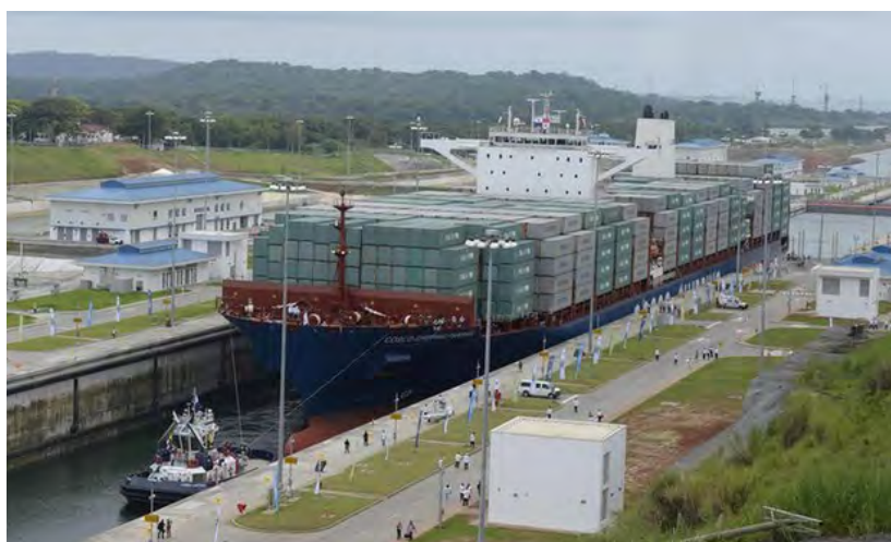
The enormous Chinese container ship MV COSCO SHIPPING PANAMA (IMO 9732606) of 300x48.25m was the first ship clearing the new Panama Canal, seen in the picture at new Aqua Clara lock, amid celebrations and fireworks. Note that at the new locks there are no locomotives, like the old passage and the ship is moved with her own power and the assisting tugs.
